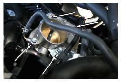
**4.** Using a 12mm socket, remove four bolts that hold the throttle body to the intake manifold.
